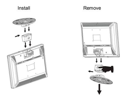
Figure 1 Installing and Removing the Swivel Base
